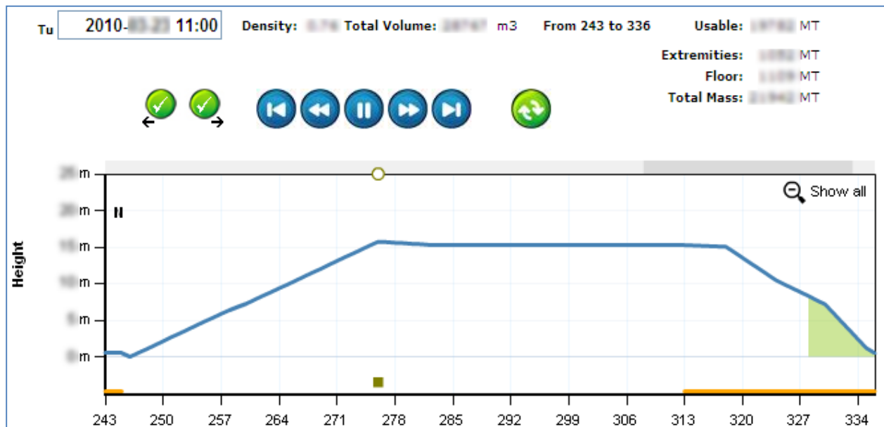
Figure 3 - If user zooms to select a region of mound, graph shows volume and mass for selection
